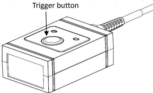
2. Press the button to decode the barcode. One beep indicates a good read.
