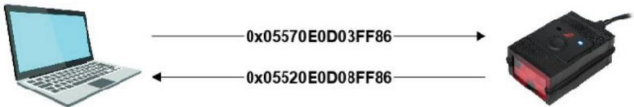
Scanner return Scan Mode data.(Data = 0x08 indicate Scan Mode is Auto Scan Mode)
