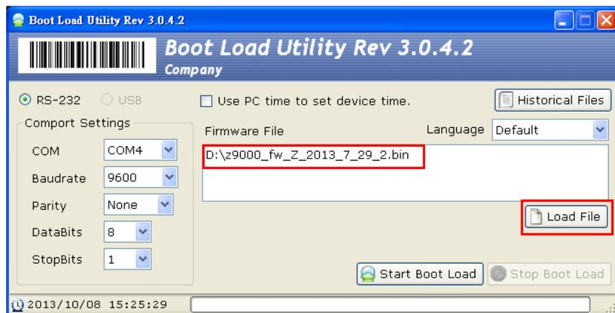
10. Select "Start Boot Load" to transfer the file to Z-9000. You will hear a beep sound when the transfer is done. The Download screen appears on the Z-9000 screen. Press ESC to exit the screen when ready.
