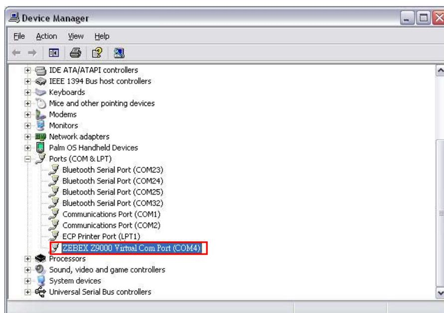
8. Select the same COM port the Z-9000 is using in Boot Load Utility.
